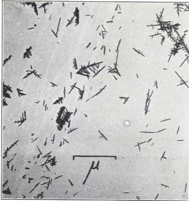
Figure 6 Electron micrograph, X19,000, of nodular rods and needles of alpha iron.
